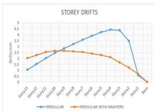
Figure 14: Storey Drifts for Irregular buildings
