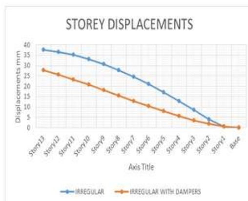
Figure 11: Storey Displacements for Irregular buildings
