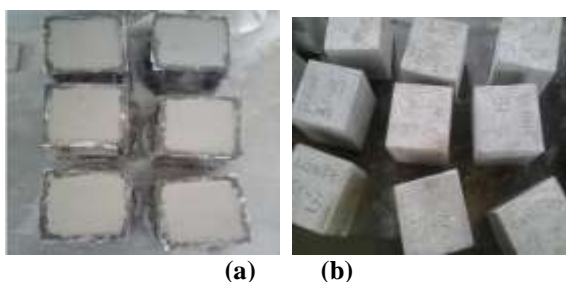
Fig-1: (a) Concrete cubes casted in the mould (b) Concrete cubes after de-moulding.
