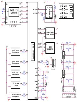
The circuit diagram of the IOT based Wearable Armed Personnel Health Condition Monitoring system is shown in the above figure. It consists of ATmega328 Microcontroller, Heart Beat Sensor, Body Temperature Sensor, MEMS Accelerometer Sensor, ESP 8266 Wi-Fi Module, Dual Band GSM MODEM, GPS receiver, LCD Display Unit and Power Supply Units.
