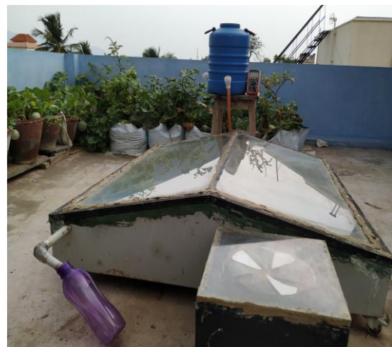
Figure.3 Schematic view of single basin double slope solar still
