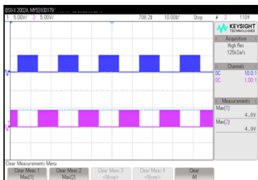
Fig.8 PWM pulse to the converter
