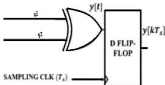
Fig.3. Architecture of XOR based phase detector
