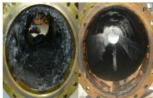
Figure 1 shows the deposition of wax in the pipeline [1].
