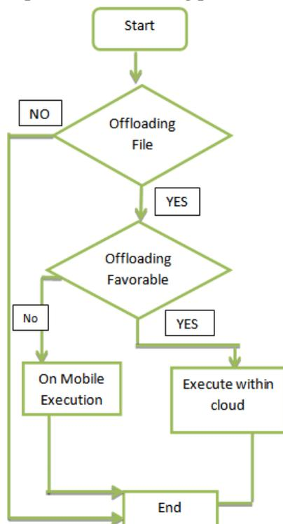
**Fig: 1.2** Computation Offloading Process
