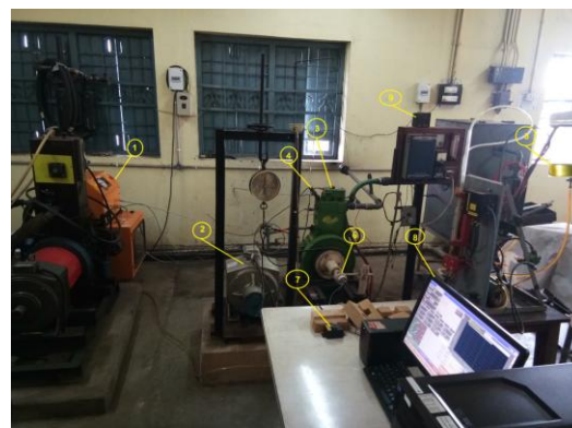
1. CRDI SYSTEM 2.EDDY CURRENT DYNAMO METER 3. DIESEL ENGINE 5.FUEL TANK 4. FUEL INJECTOR 6. CRANK ANGLE ENCODER 7. INJECTION DURATION CONTROLOR 8. COMPUTER INTERFACED TO CRDI SYSTEM 9. EXHAUST TEMPERATURE INDICATOR
