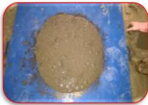
Fig 3 Slump Flow of Self-Compacting FDHP Concrete
