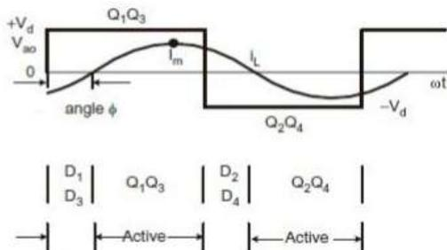
Fig.5 Load voltage and current waveform
