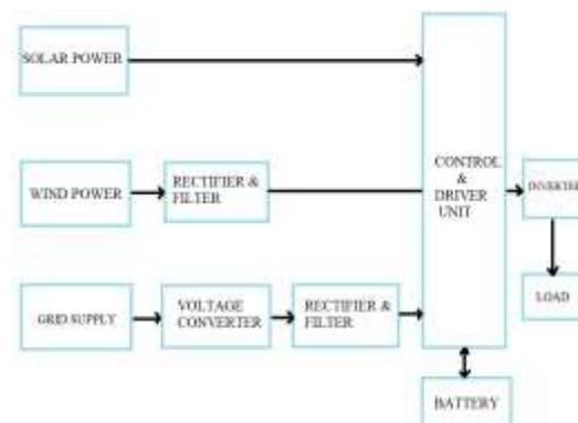
Fig.1 Block diagram of hybrid energy system
