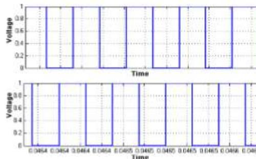
Fig.7 Pulses for Q1, Q2 & Q3,Q4
