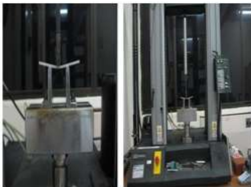
Fig 2.2: 3 point bending test of composites, Specimen loaded in Universal Testing Machine
