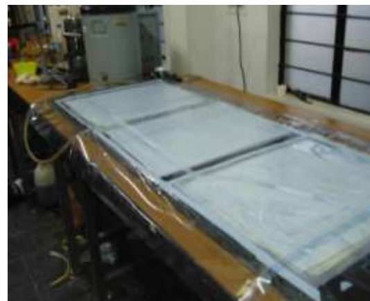
Fig-2.1: Moulded laminates under vaccum bagging process
