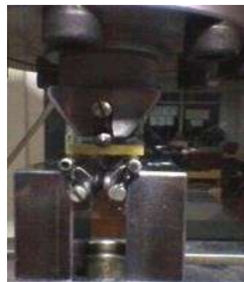
Fig 2.3: ILSS test of composites, Specimen loaded in Universal Testing Machine
