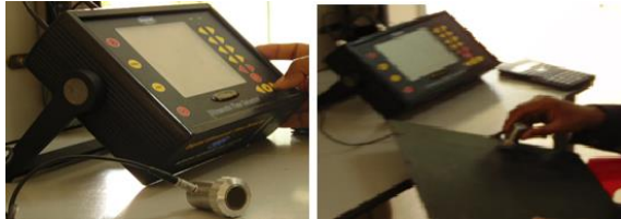
Fig-3.1. Ultrasonic B-scan on composite laminates
