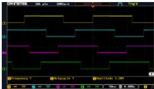
Figure 19.- Shots Inverter Switches single phase AC/AC
