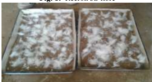
Figure 2: Recron 3S Fibre plus soil
