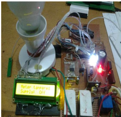
Figure 7: GSM based Energy Meter Showing 'Meter tampered' when tried to be bypass.
