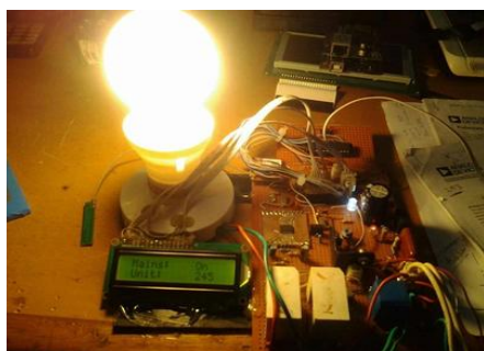
Figure 5: GSM Based Energy Meter Showing Mains 'ON' and Unit Balance.
