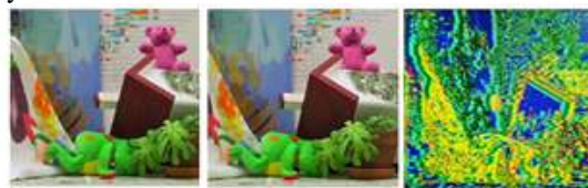
Fig.8 Proposed system input and output images (Teddy) (a) left images (b) right images (c) disparity images
