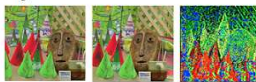
Fig.9 Proposed system input and output images (Cones) (a) left images (b) right images (c) disparity images
