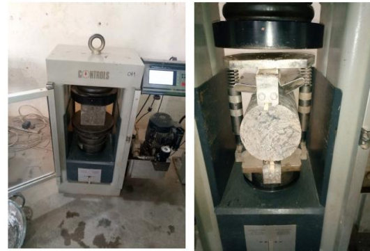
Figure 1 compression and split tensile strengths setup
