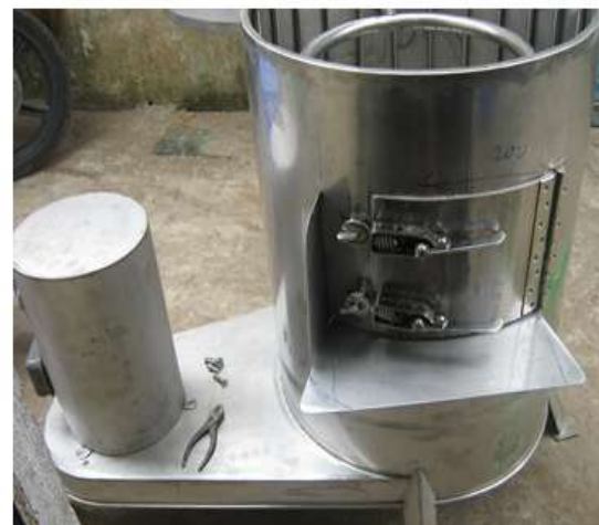
Figure 6: The pig stomach washing/cleaning machine after manufacturing in the practice
