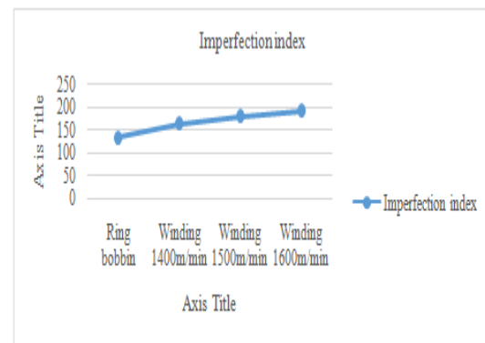
Fig 4: Effect of winding speed on imperfection index.
