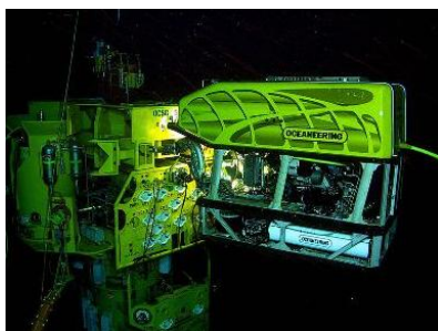
Figure15. An ROV equipped with a modern technology lighting system and video camera (Marine Technology)
