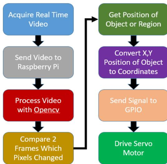
Fig. 4 Block Diagram of Entire System
