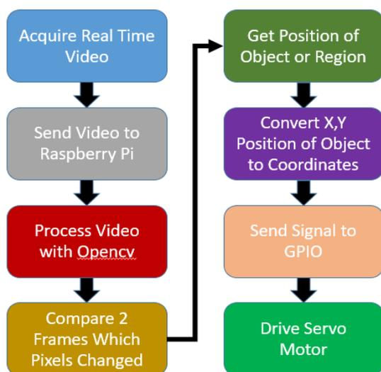
Fig. 4 Block Diagram of Entire System
