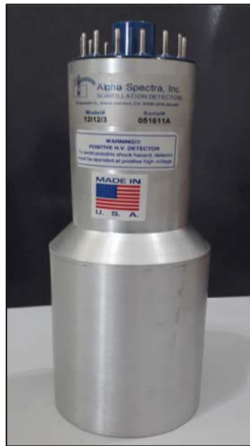
Fig. 1 – Sodium Iodide scintillator and photomultiplier used in this gamma radiation measurements, (Aware Electronics, INC, USA).
