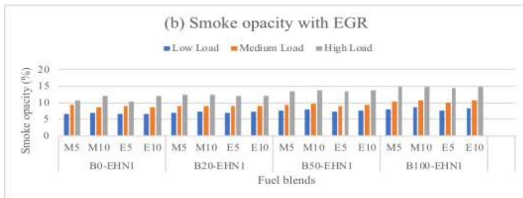
Figure 9: Smoke emissions of different fuel blends (a) without EGR (b) with EGR
