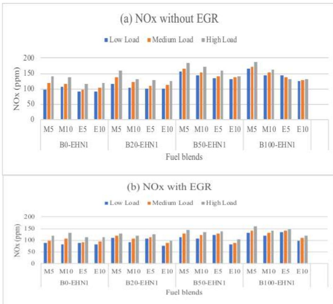
Figure 8: NOx emissions of different fuel blends (a) without EGR (b) with EGR
