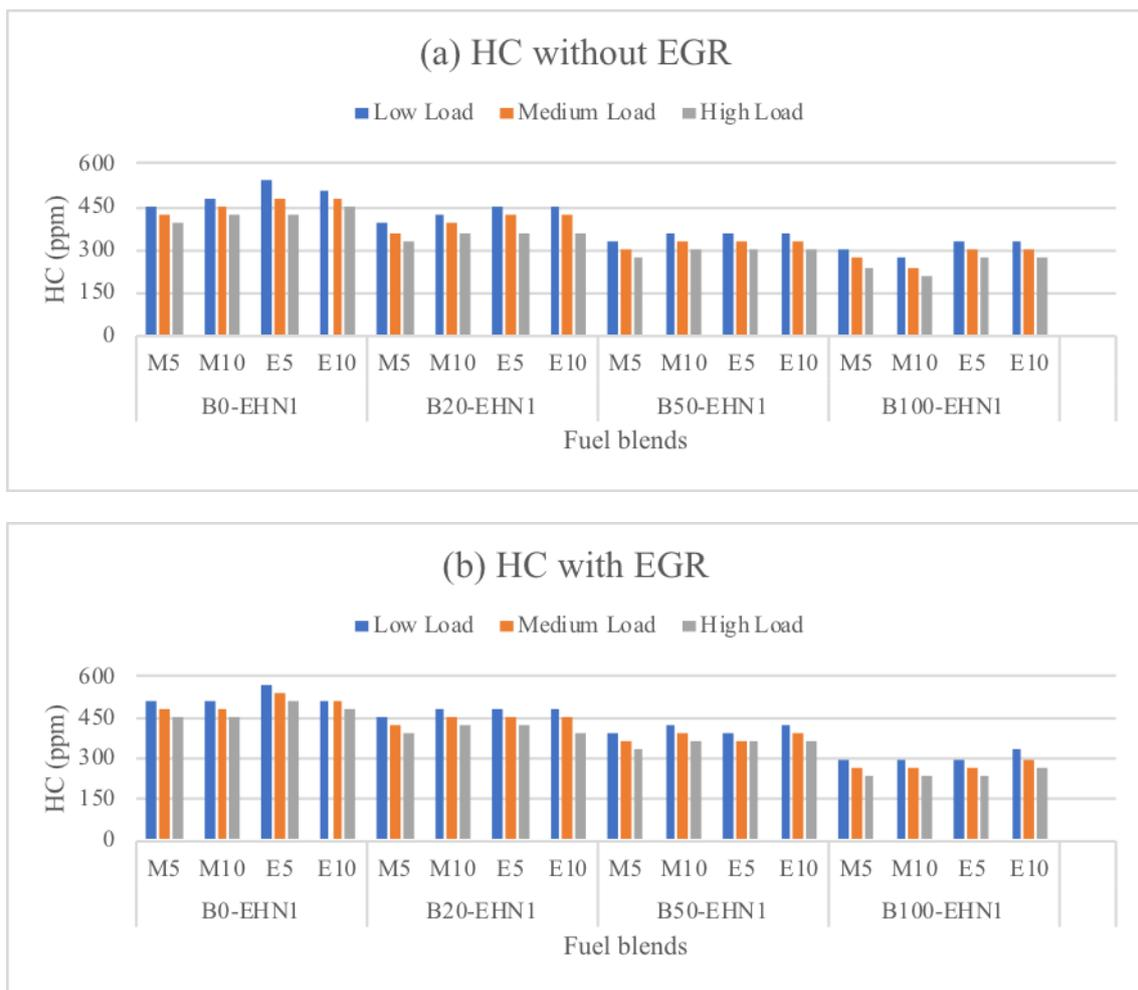
**Figure 7:** HC emissions of different fuel blends (a) without EGR (b) with EGR
