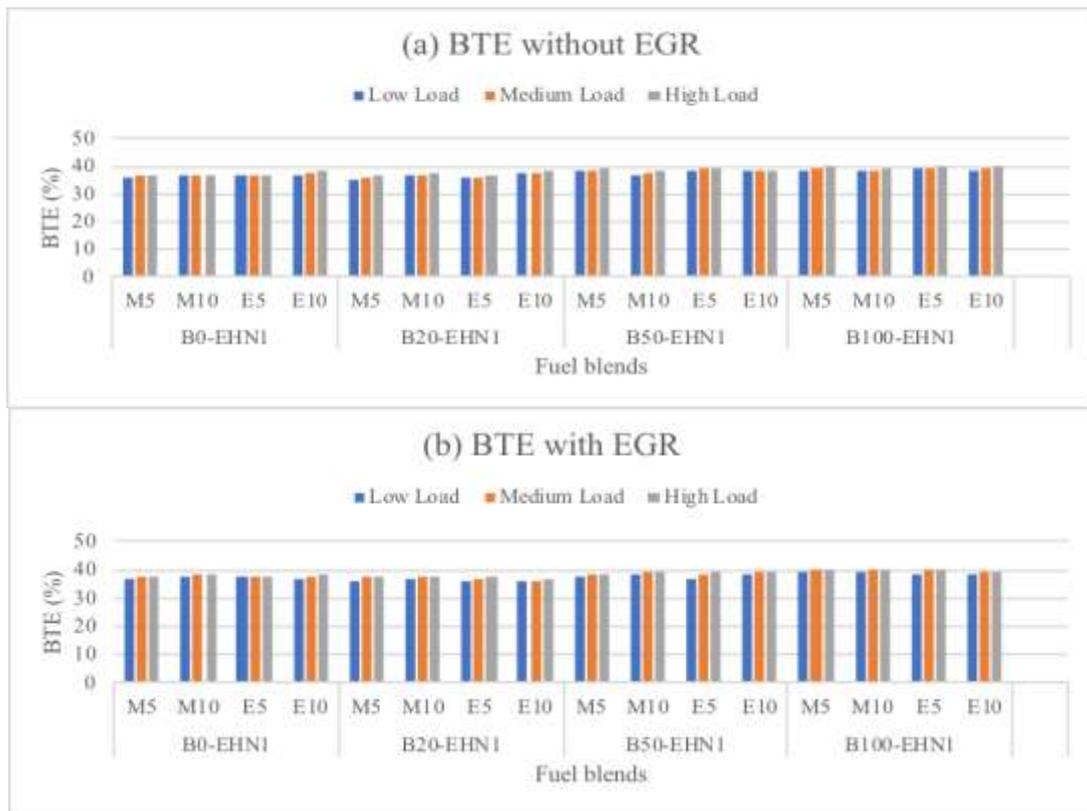
**Figure 4:** BTE of different fuel blends (a) without EGR (b) with EGR
