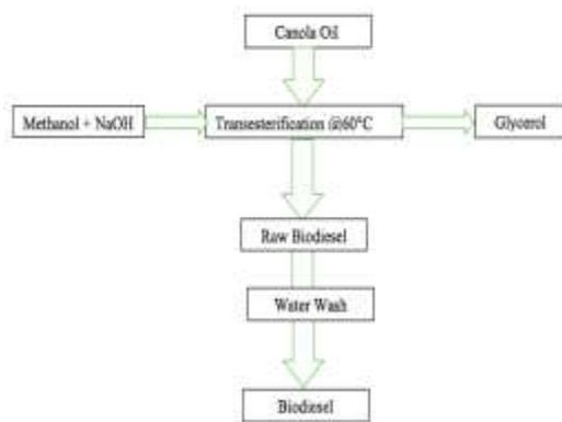
**Fig. 1:** Production of biodiesel through transesterification process from canola oil
