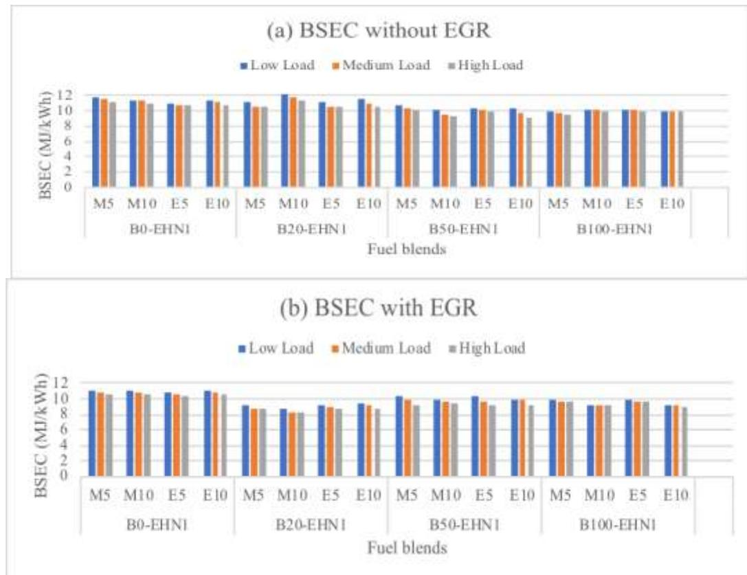
**Figure 5:** BSEC of different fuel blends at (a) without EGR (b) with EGR
