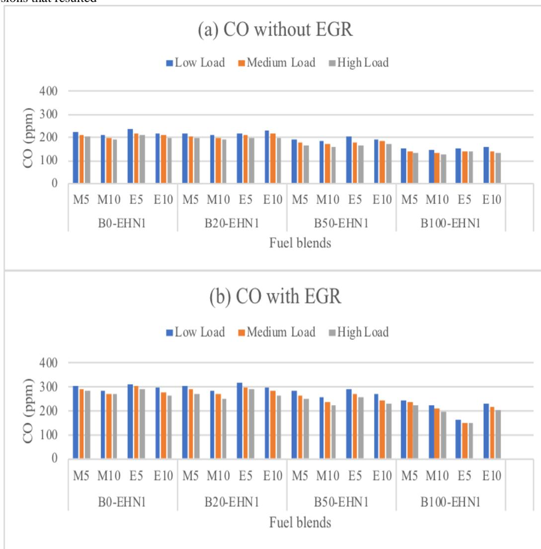
**Figure 6:** CO emissions of different fuel blends (a) without EGR (b) with EGR
