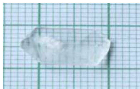
Figure.2 (b) L-Arginine doped KHP (LA-KHP) single crystal
