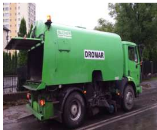
Fig. 1. The container is designed to collect impurities in self-propelled vacuum sweeper
