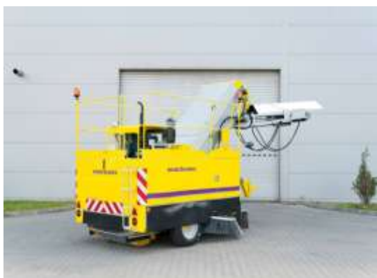
Fig. 2. An elevator sweeper, adapted for towing a tipper truck
