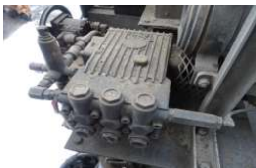
Fig. 10. WS-104 pump, mounted on Bucher Schörling sweeper, forcing water into the PM10 system
