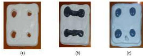
Figure 8 Directgelcast printing of multi-layer materials in the following sequence (a) AlN interposer, (b) Mo conducting line, (c) AlN interposer on top of Mo line.
