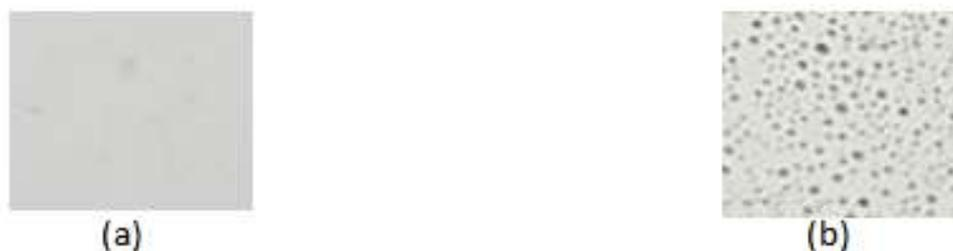
**Figure 4** Optical image of AlN sintered sample with the slurry prepared using (a) mortar and pestle for 20 minutes and (b) ball mill at 150rpm for 1 hour.
