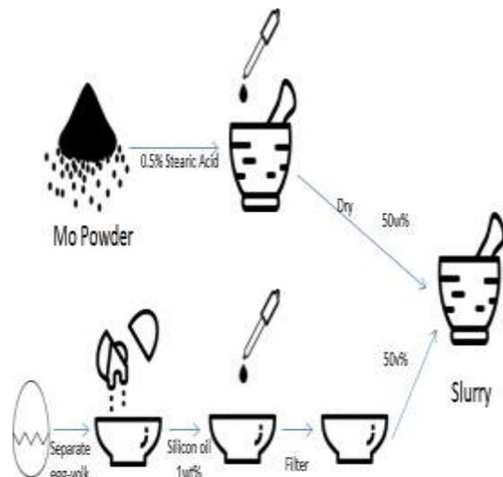
Figure 2 Preparation of Molybdenum slurry.
