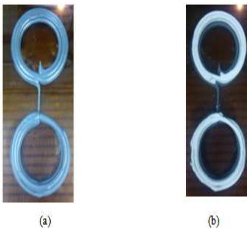
Figure 7 Direct gelcast printing of multi-material a) Mo, b) AlN on Mo.
