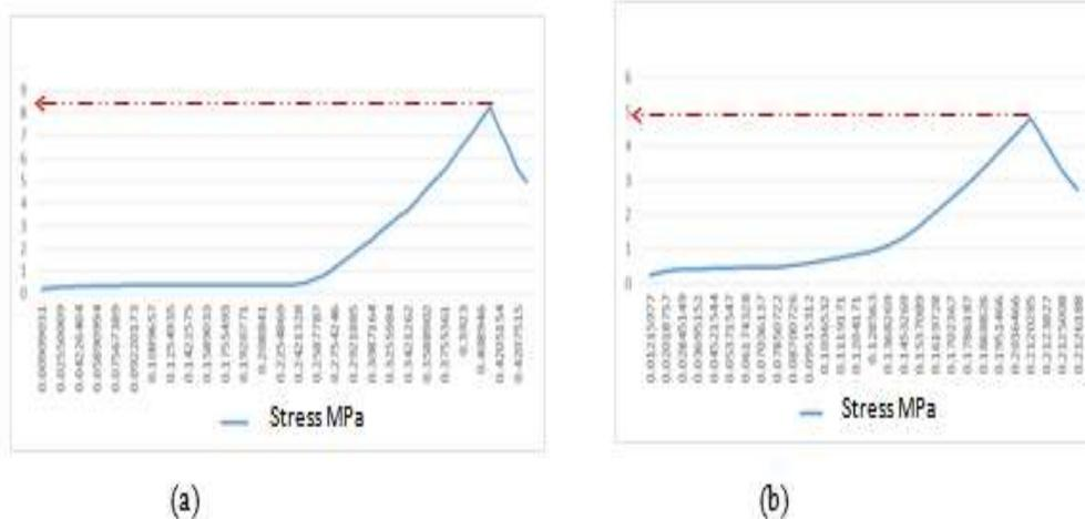
**Figure 3** Flexural strength measurement of (a) slurry prepared using a mortar and pestle (20 min) and (b) slurry prepared using a ball mill (150 rpm for 1 hour).
