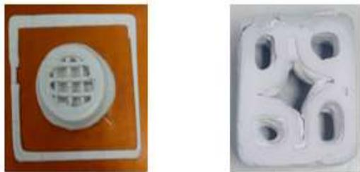
Figure 6 3D structures of AlN.
