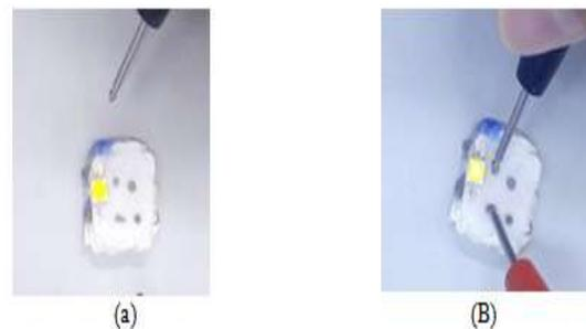
Figure 9 Functional interposer with AlN with embedded Molybdenum conducting line (a) before applying current (b) LED turn on when applying DC current.
