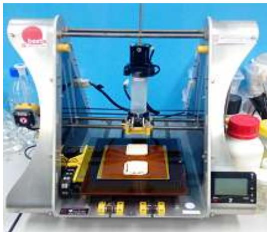
Figure3 Thick paste extruder (ZMorph 2.0).
