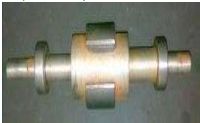
Fig.3. Mounted magnet on the rotor shaft.
