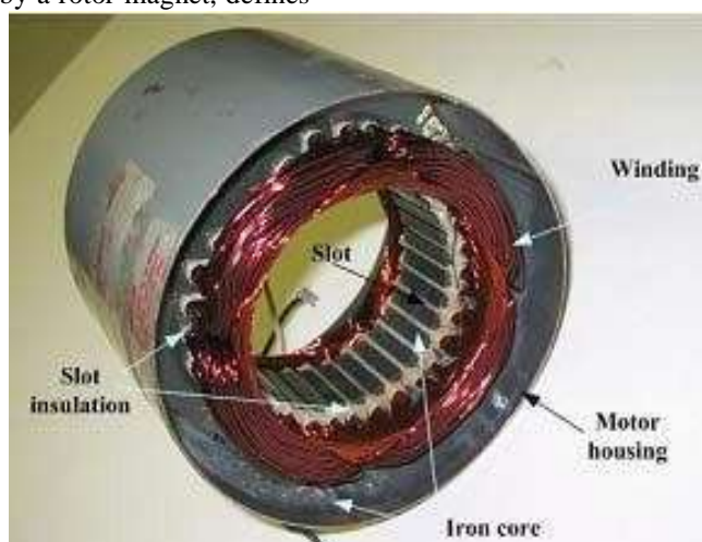
Fig.2. Stator Case with Winding.
