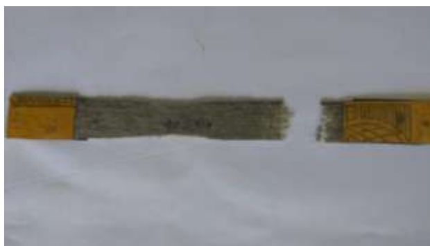
Figure13: Specimen of flyash content of 40% after testing
