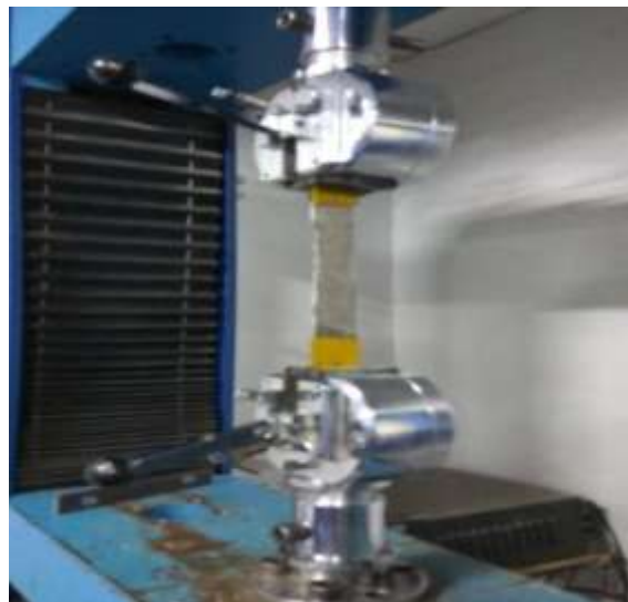
Figure 12: Specimen on UTM during tensile test
