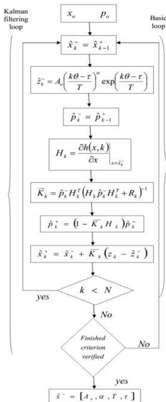
Fig. 2 Flow diagram that specifies the application of DEKF to ultrasonic echoes
