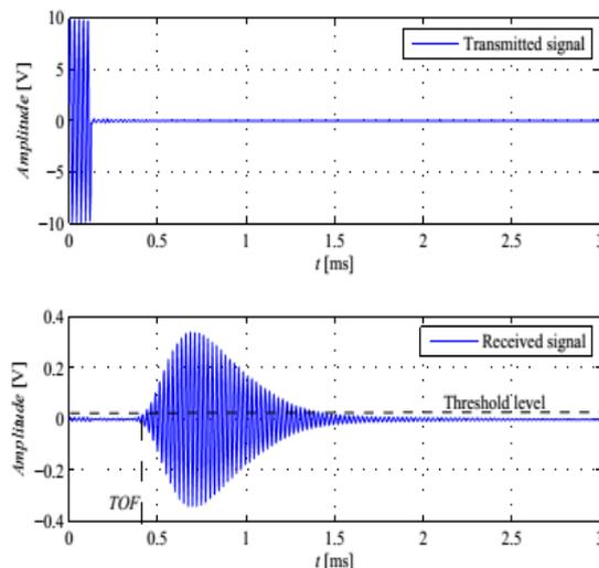
Fig.4 TOF estimation by Threshold method
