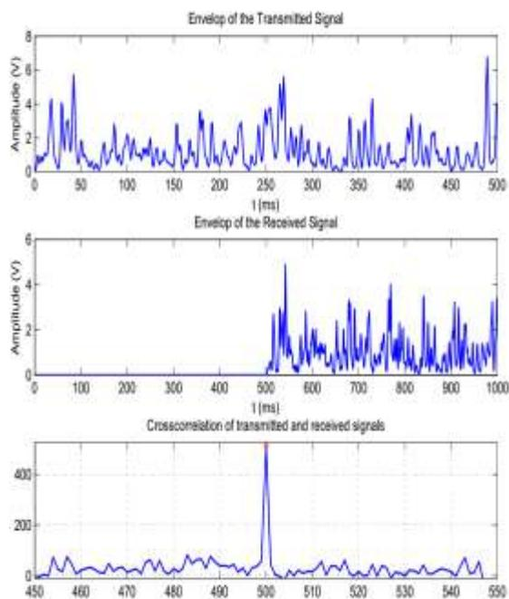
**Fig.6 TOF estimation by Cross Correlation estimation**
