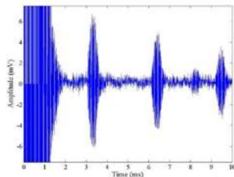
**Fig.7 Original Ultrasonic signal digitized at 250 KS/S with multiple Echoes**
