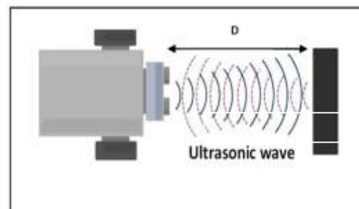
Fig. 1 Illustration of Ultrasonic Ranging
