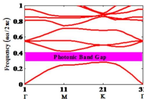
Figure 6. Band diagram for a 2-D structure showing the photonic bandgap in polarization TM for the material GaAs. The diagrams represents propagation of the wave vector in the  $x$ -direction, giving the points of high symmetry  $\Gamma$ , M, K in the first Brillouin zone. On the  $y$ -axis are plotted the frequencies of the calculated modes. In the TM mode, there is a forbidden band of width  $0.1367\mu\text{m}$  for the ratio  $r/a = 0.2$ .
