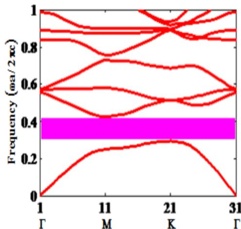
**Figure 7. Band diagram for a 2-D structure showing the photonic bandgap in polarization TM for the sapphire (Al<sub>2</sub>O<sub>3</sub>) material. The bandwidth is equal to 0.1331μm. It is slightly lower than that observed with the gallium arsenide (GaAs) material. In the TE mode, we do not observe any forbidden band.**
