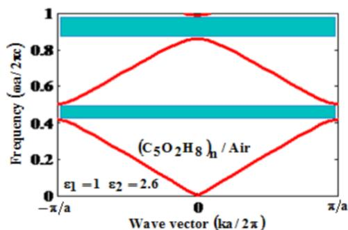
Figure 5. Dispersion relation for the Plexiglas  $(\text{C}_5\text{O}_2\text{H}_8)_n$  material with permittivity  $\epsilon_a = 2.6$  for the same values of the coefficient  $r/a$  as in Fig. 3. Two photonic bands are observed with a greatest bandwidth of  $0.11\mu\text{m}$  obtained for  $r/a = 0.1$ . The number of elements is the same as in Figures 3 and 4.
