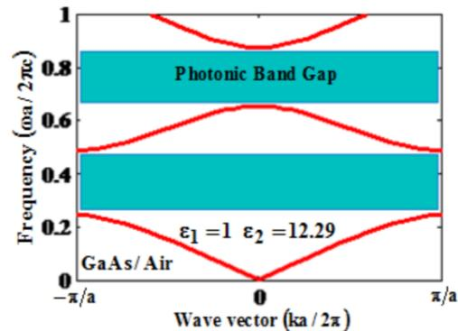
Figure 3. The photonic band structures for a 1-D photonic crystal. This relation is presented for the GaAs material of permittivity  $\epsilon_a = 12.29$  and the coefficient  $r/a$  was varied over the range from 0.1 to 0.3, with  $a = 0.775 \mu\text{m}$ . The number of elements is  $N = 5$ . Two photonic bands are counted and the greatest bandwidth obtained is  $0.24 \mu\text{m}$  with  $r/a = 0.1$ .
