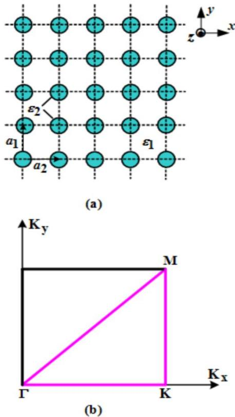
Figure 2. (a) Structure of a 2-D photonic crystal and (b) the corresponding Brillouin zone (purple line).  $\epsilon_1$  and  $\epsilon_2$  are constant permittivities of the first and second materials, respectively.  $a_1$  and  $a_2$  are the basis vectors of the network, in the  $y$  and  $x$ -directions, respectively.
