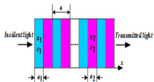
**Figure 1. Geometry of a 1-D photonic crystal structure.  $\epsilon_1$  and  $\epsilon_2$  are constant permittivities of the first and second materials, respectively.  $n_1$  and  $n_2$  are the refractive index constants of the first and second materials, respectively.  $a$  is the periodic spacing.**
