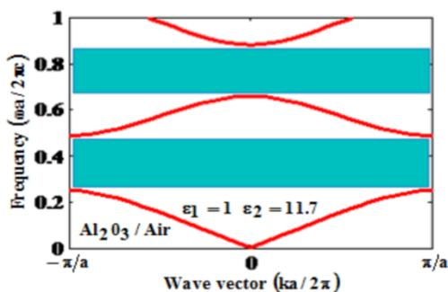
Figure 4. Dispersion relation for the  $\text{Al}_2\text{O}_3$  material with permittivity  $\epsilon_a = 11.7$  for the same values of the coefficient  $r/a$  as in Fig. 3. Two photonic bands are observed with a greatest bandwidth of  $0.23\mu\text{m}$  obtained for  $r/a = 0.1$ . The number of elements is the same as in Figure 3.
