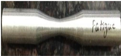
Figure 1: Fatigue Test Specimen
