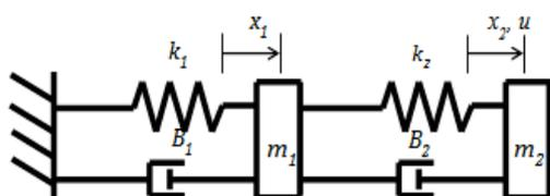
Figure 2. Double Mass Spring Damper System
