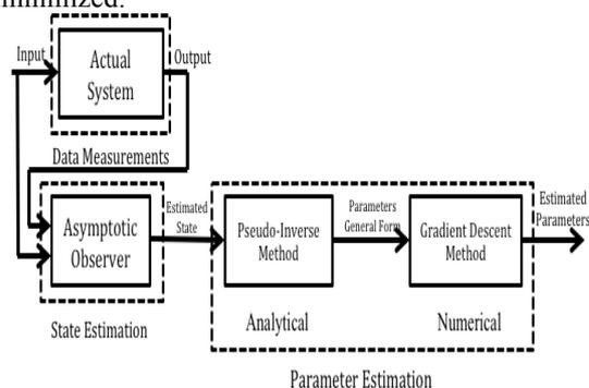
Figure 1. Parameter Identification Flow Chart
