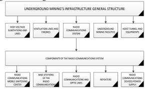
Fig. 1.Underground mining infrastrucure and radio communications system's general structure
