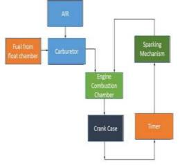
Fig 3.1: Block diagram of conventional two stroke
