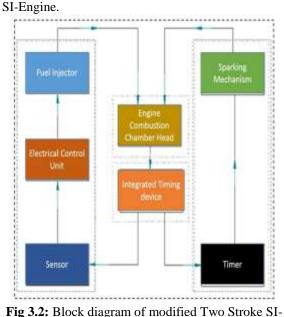
g 3.2: Block diagram of modified Two Stroke SI Engine (DFI-System)
