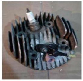
Fig 3.4 Modified DFI 2 stroke engine
