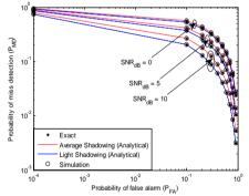
Fig. 2 Complementary ROC curves for light and average shadowing
