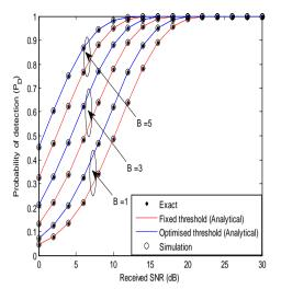
Fig. 7 Probability of detection against received SNR with fixed and optimized threshold
