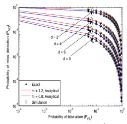
Fig. 4 CROC curves for different d with no diversity (m = 0.8, 1.2, SNR = 0 dB)
