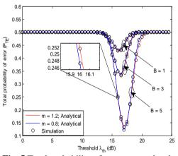
Fig. 5 Total probability of error verses threshold for number of diversity branches
