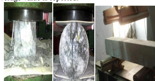
Fig. 3 (a) Failure of cube under compression, (b) split tension, (c) flexural test setup
