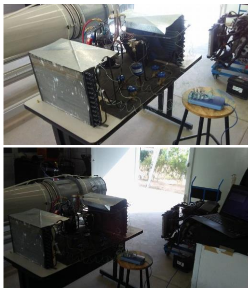
Fig.6. Instrumented reverse cycle machine.
