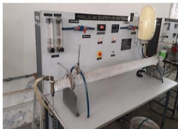
Fig. 5. Parallel and Counter flow heat exchanger for experimentation
