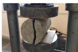
Fig. 1a. Split Tensile Test on Cylinder
