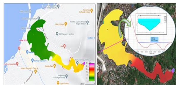
Fig 10. 2D Model of Way Ruhu River flow and wide cross section of inundation plain
