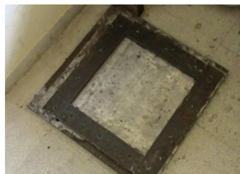
Fig 3. Mould for casting the composite
