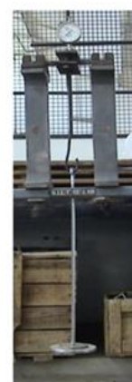
Fig 7. Test Setup for flexural test
