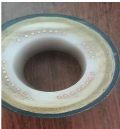
FIG. 3.6 Power line layout in the novel-flexible long tube in narrow-band carrier communication system
