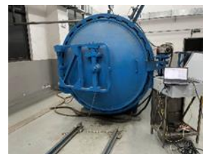
(b) Test diagram of carrier module in an 80°C incubator
