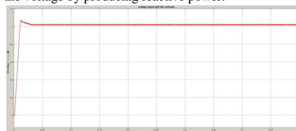
Fig 5.8 Voltage profile at the end of the busbar with using GA controllers.
