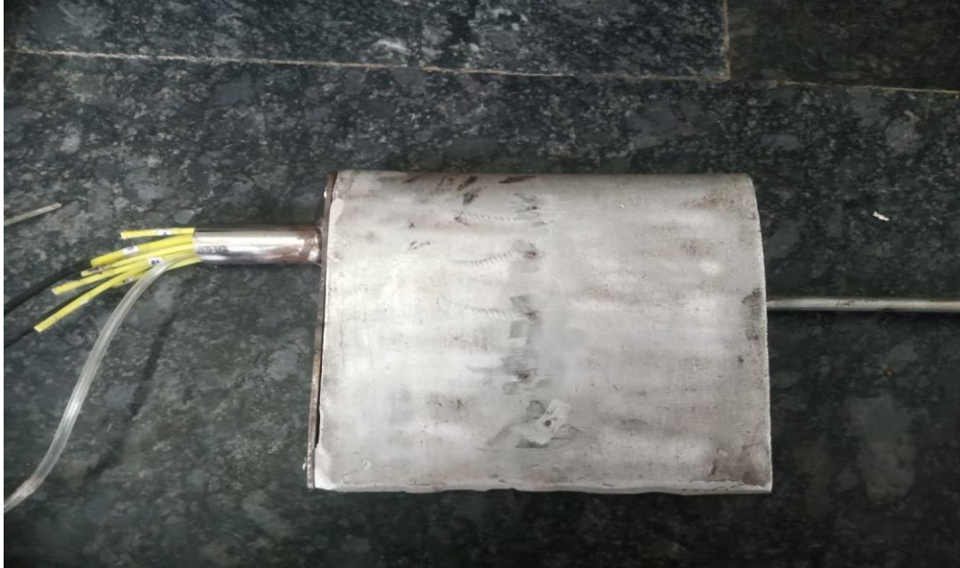
Fig.11: NACA 0012 AEROFOIL ARRANGMENT WITH PRESSURE TAPS
