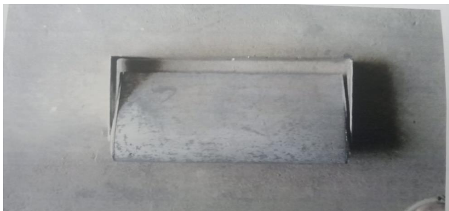
Fig.5: Aerofoil model with clamping device.
