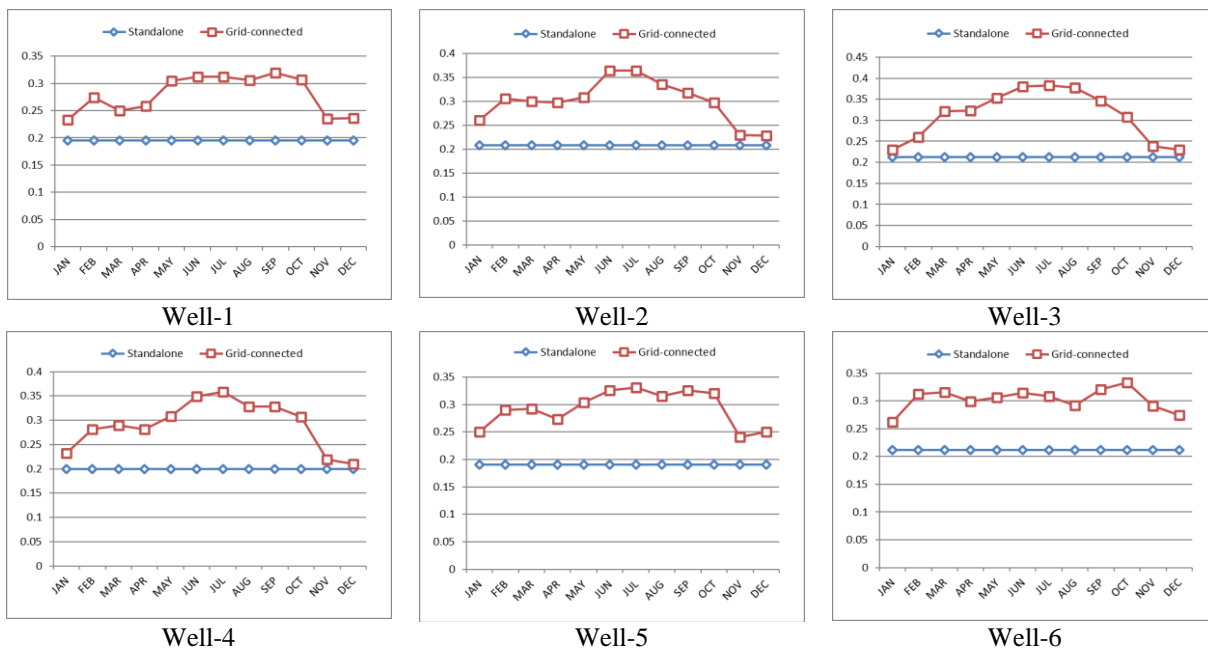
Figure 15: Capacity Factor (CF) at using one-axis tracking system for both stand-alone and grid-connected cases
