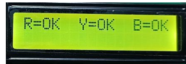
Fig.7: Phase Fault Detection
