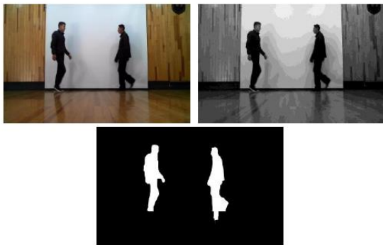
Fig. 18 This image shows two pedestrians walking in opposite directions in the auditorium with wooden stave and wooden walls, a white screen was placed in order to obtain a good segmentation.
