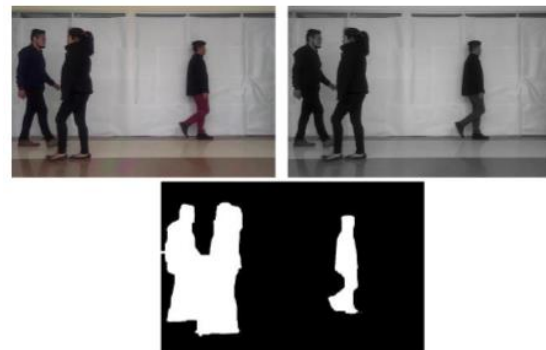
Fig. 16 It can be seen the segmented result of three pedestrians walking in the 3rd floor corridor of the graduate building, the original RGB, grayscale and binarized segmented images are shown.
