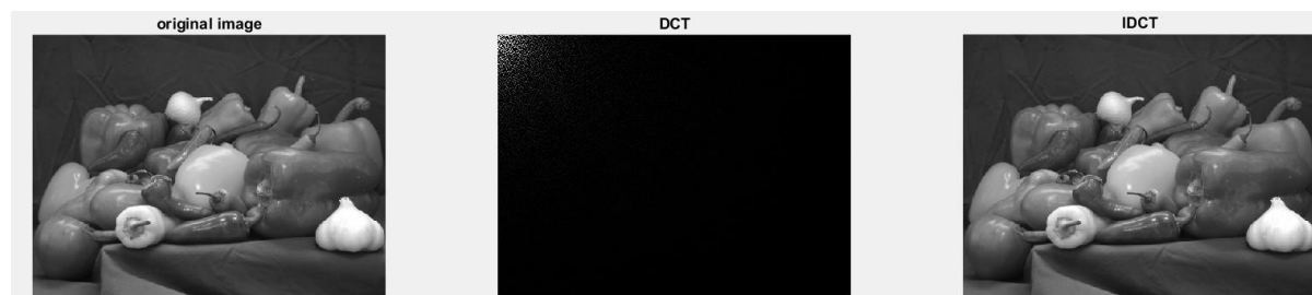
Fig:1 Energy concentrated in left corner shows the compaction property of DCT
