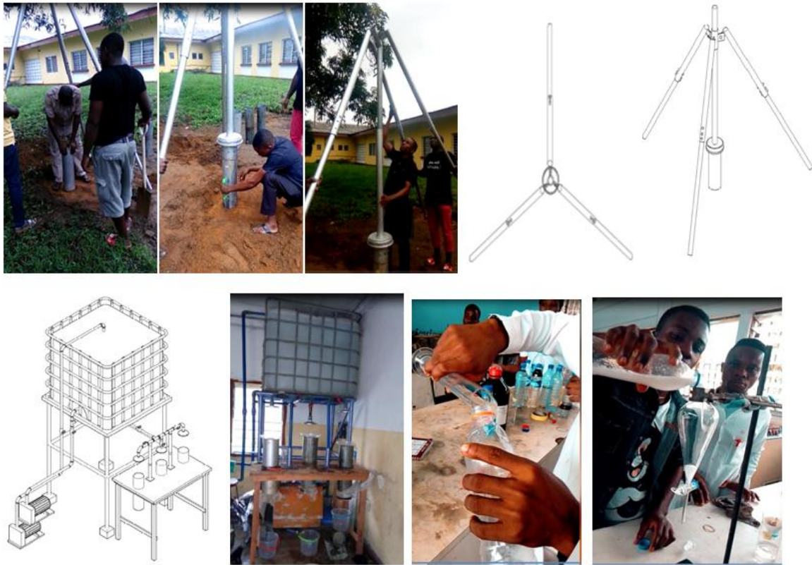
Plate 1. Installation of the fabricated auger rig undisturbed soil collector before soil collection.
